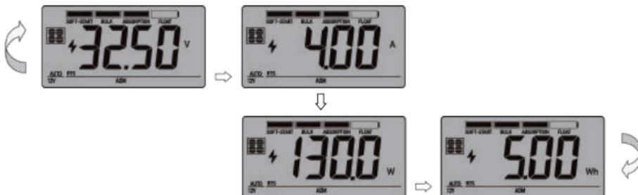
Press **BATT / - button** in sequence, the LCD will display in turn with battery voltage, charging current, charged capacity (Amp-hour) and battery temperature (if external temperature sensor connected)
