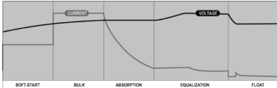
For Lithium battery (LCO, LFP, LTO battery)
