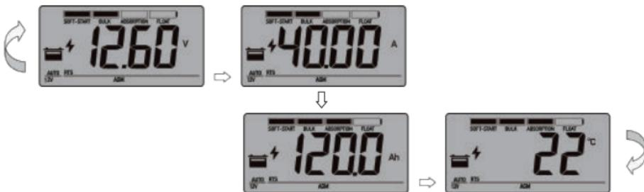
The users also can read the battery voltage as degree centigrade or Fahrenheit degree by pressing **SET UP button** for converting.
