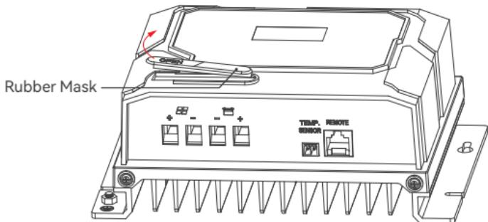
Please do not reverse the connections with the solar panel and battery when installed the cables.
