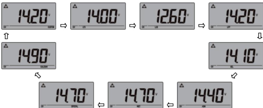
Press the **SET UP button** again, the selected battery type will be solidly On and confirmed.
