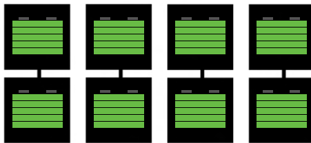
Example 24V System (8x 12v Batteries, Wired in Series to 24V Series Parallel System)
