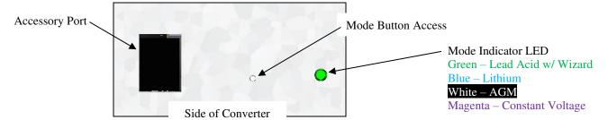
Press and hold the MODE BUTTON for at least 3 seconds until the LED changed color. Continue to depress button until the desire battery type is selected.
