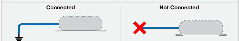
Figure 10: Connecting the BLUE wire to solar panel
