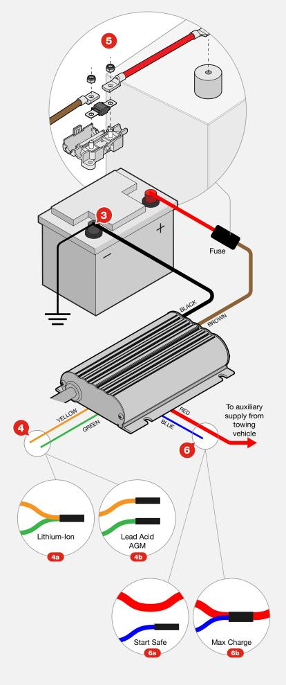
This is a generic installation for illustration purposes. Read the BCDC1212T instruction manual for further installation information. For further assistance with your BCDC installation, contact REDARC at power@redarcelectronics.com
