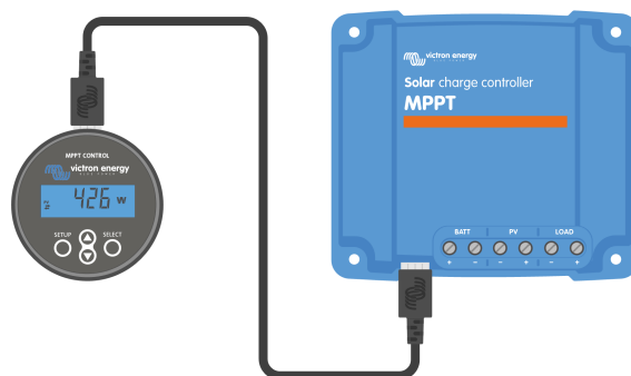
Connect the display to the solar charger via a VE.Direct cable
