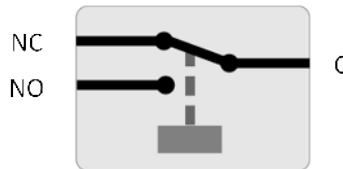
Internal operation of the programmable relay
