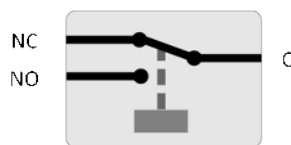
Relay configuration (not energised).
