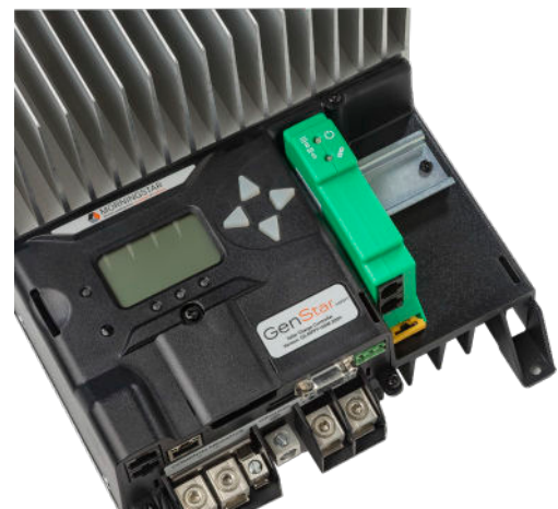
ReadyBMS installed in a GenStar MPPT charger
