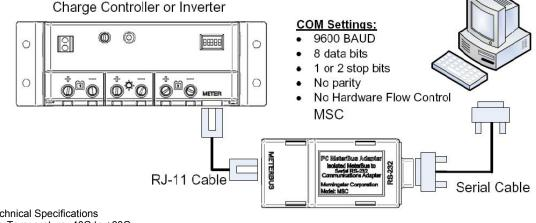
Other Technical Specifications Operating Temperature -40C to +60C Storage Temperature -55C to +80C Humidity 100% N.C. Enclosure IP20 Dimensions 72 x 35 x 22mm 2.83 x 1.37 x 0.87 inches Weight 35 g (1.23 oz)
