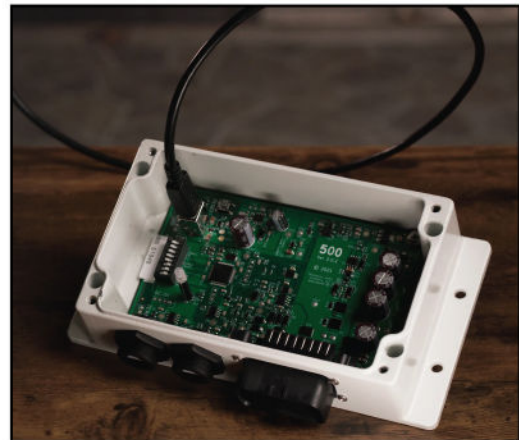
Figure 6 - Type B USB cable connected
