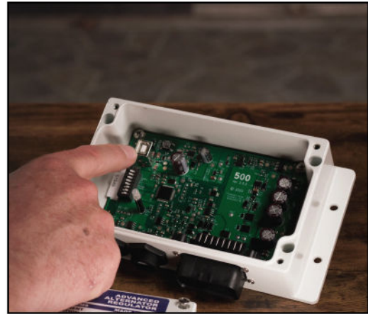
Figure 5 - Type B USB connector & reset button
