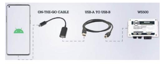
Transferring a configuration file to a Wakespeed regulator using the Wakespeed Mobile App on an Android device.
