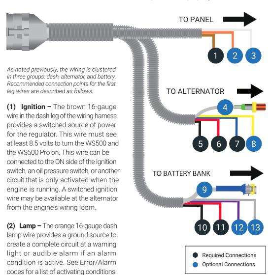
(3) Function In – The white 16-gauge Function In can be configured to provide a number of custom controls which can be activated by connecting the wire to >8.5VDC+ via a toggle or other ON/OFF type switch. In default mode, the Function In mode will enable equalize mode when the regulator is configured for lead acid batteries. When the WS500 WS500 and WS500 Pro are configured for LiFePO<sub>4</sub> batteries (see DIP switch instructions), Function In will force the system to float.
