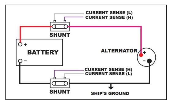
NOTE: DIAGRAM IS INTENDED TO INDICATE PLACEMENT OF CURRENT SENSE WIRES BASED ON SHUNT LOCATION. ONLY ONE SHUNT IS REQUIRED FOR REGULATOR OPERATION.
