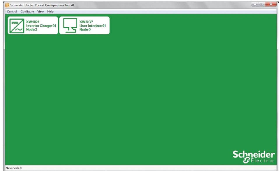
NOTE: Only the XW Pro unit to be calibrated (in step 6) should appear here. If other XW Pro units are appearing, then these units must be turned off via the AC and DC breakers. Repeat step 5 for these units.
