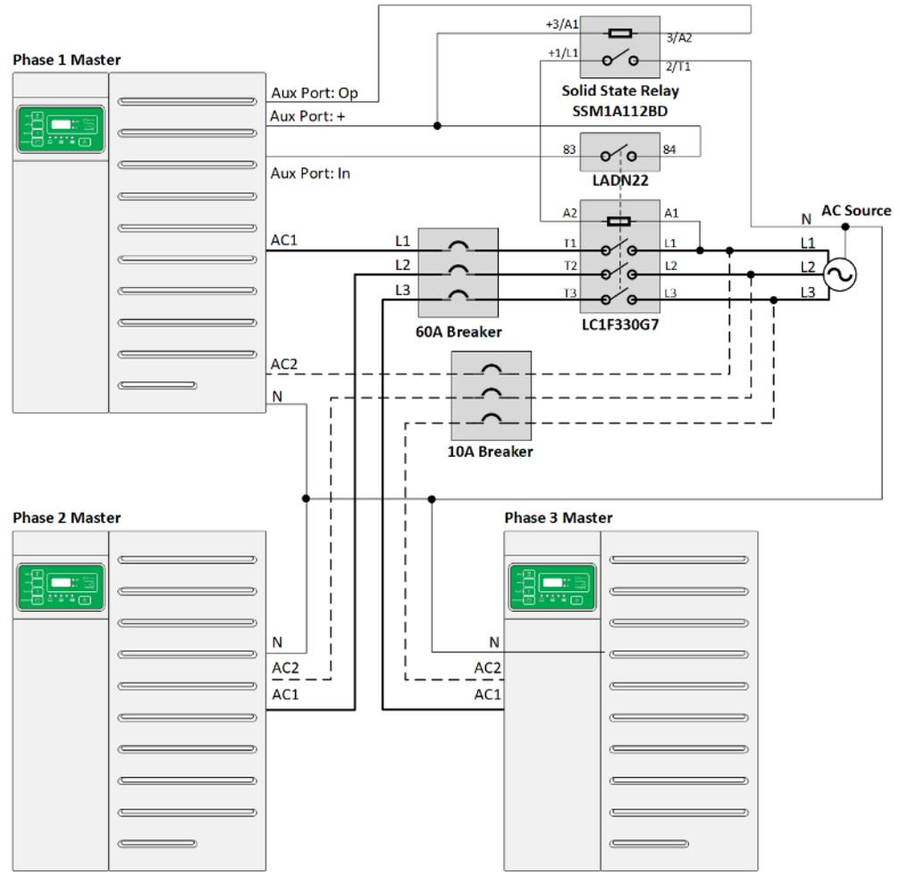
For larger three phase systems, up to two 3-phase clusters (6 XW Pro units) can be connected in parallel, limited by the synchronization limits of the inverters.
