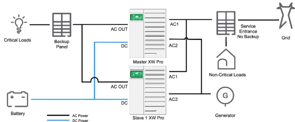
AC and DC-coupled sources are not represented for simplicity. However, they can be integrated into the system as shown in *Figure 9 on page 28*.
