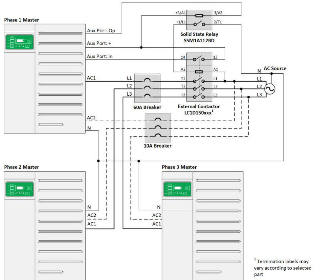
Figure 18 External contactor AUX port and mains connection diagram (three-phase 120/208V configuration shown)
