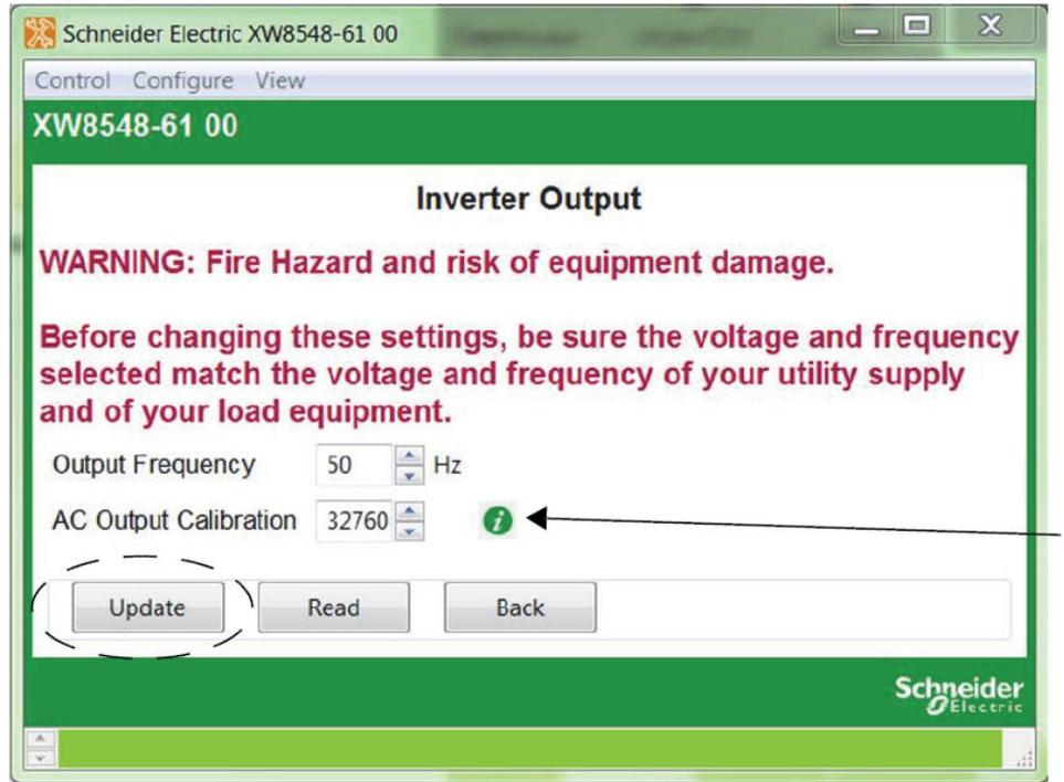
NOTE: To make the changes permanent, adjust the **AC Output Calibration** scaler value and the **Output Voltage** change will become permanent after the unit resets.
