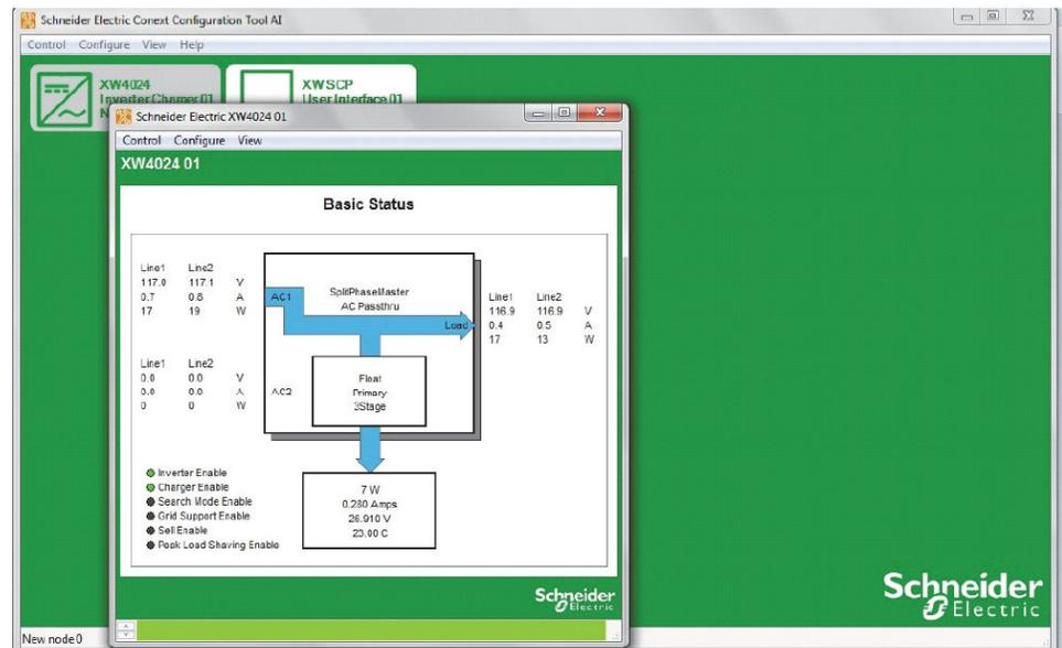
10. Go to **Configure -> Inverter -> Inverter Output**.
