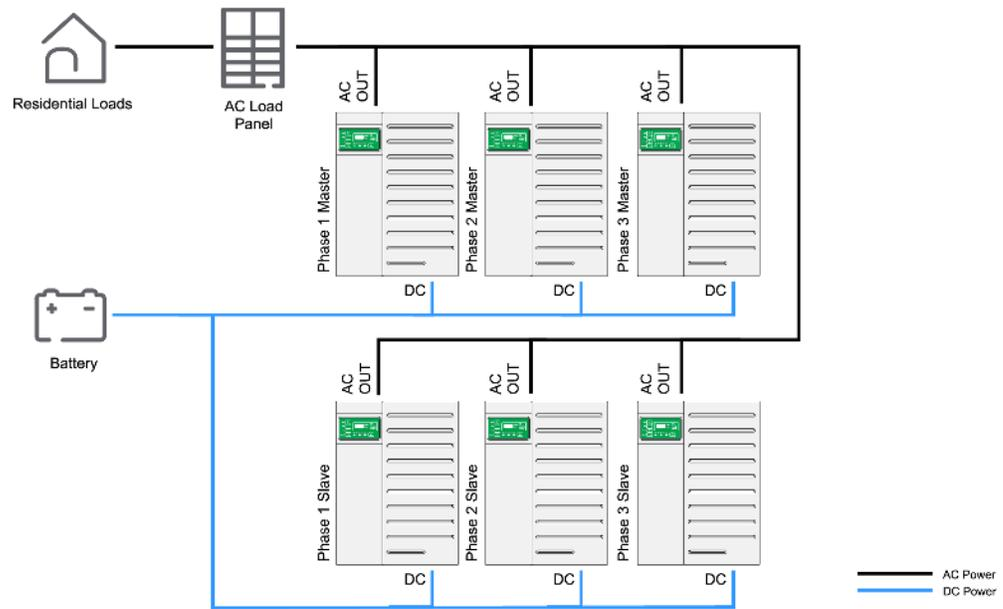
If no AC source is connected at the input of the XW Pro, then the internal relay current limitation is no longer in place for the system. As a result, associated power ratings and the supported feature by configuration in Figure 19 are listed in Table 14. The XW Pro 8548 and XW Pro 6848 models can support up to two three-phase clusters (6 units) in this configuration based on the synchronization limits of the inverter.
