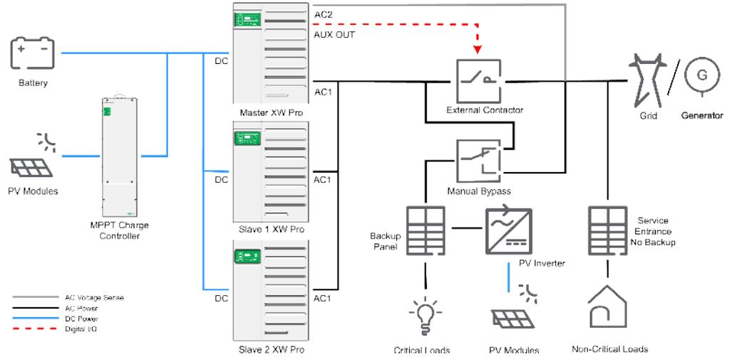
**NOTE:** For external contactor configurations, it is recommended to install a manual bypass switch to connect backup loads to the grid in case of maintenance procedures or issues with the energy storage system. An appropriately-rated SquareD or Schneider Electric ComPact INS/INV series double throw switch can be used.
