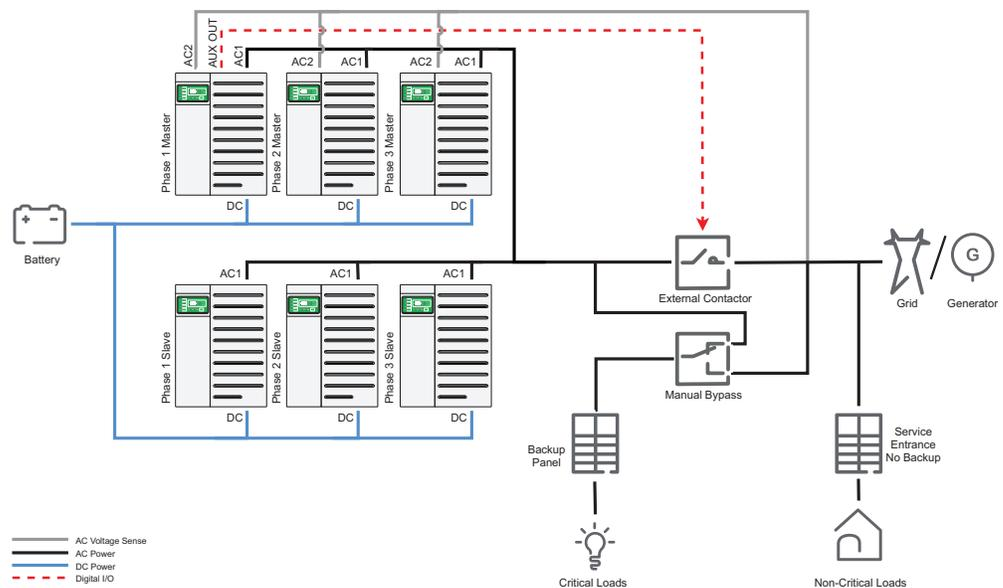
It is recommended to install a manual bypass switch to connect backup loads to the grid in case of maintenance procedures or issues with the energy storage system. An appropriately-rated SquareD or Schneider Electric ComPact INS/INV series double throw switch can be used.
