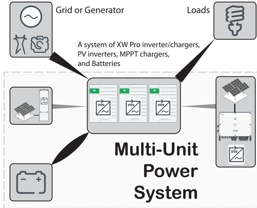
Multi-Unit Power System can be used as a grid-tie power backup equipment or as primary power sources for off-grid sites. They may or may not have solar energy harvest capability or other alternate energy sources.
