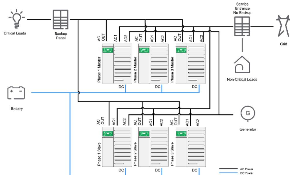
The XW Pro can be used for 3-phase systems by installing clusters of three inverters, with one inverter per phase. In configurations similar to the one displayed in *Figure 15* where no external contactor is being used, the system is subject to the 60 A limit of the internal relay. As a result, associated power ratings and the supported feature are listed in *Table 10* and *Table 11*.
