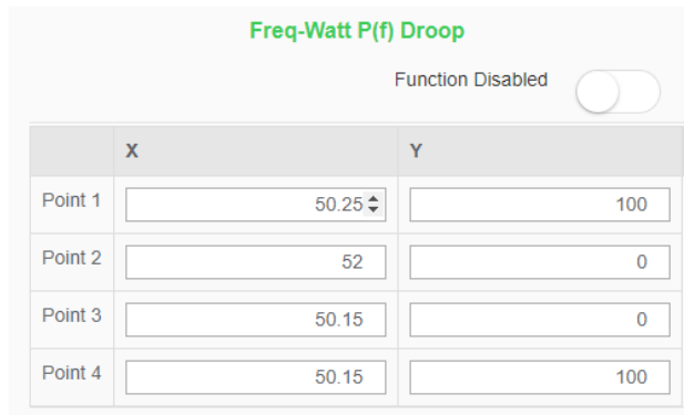
Figure 6 Disabling grid code frequency shifting in Conext Gateway GUI
