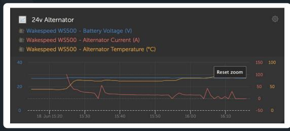
VRM custom widget showing WS500 voltage, current and temperature
