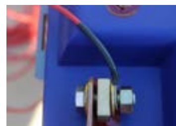
Figure 12: Bolt, washer, battery cable, positive terminal, washer, 5/16" heat-enable wire, nylok
