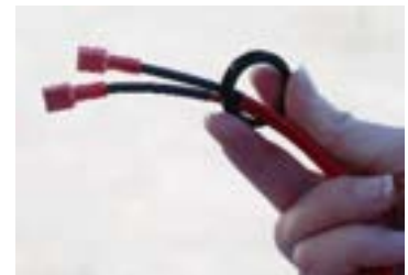
Figure 9: Heat Battery Kit harness through plastic nut
