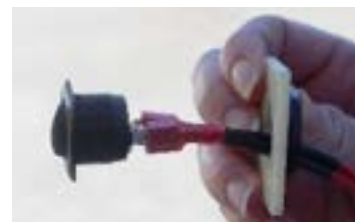
Figure 10: Heat Battery Kit harness connected to rocker plastic nut from rocker switch
