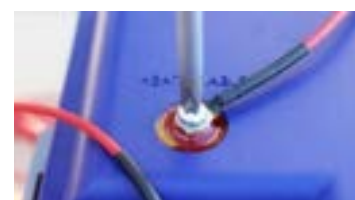
Figure 13: #8 ring terminal onto the heater enable post
