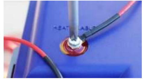
Figure 13: #8 ring terminal onto the heater enable post
