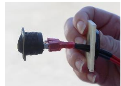
Figure 10: Heat Battery Kit harness connected to rocker plastic nut from rocker switch
