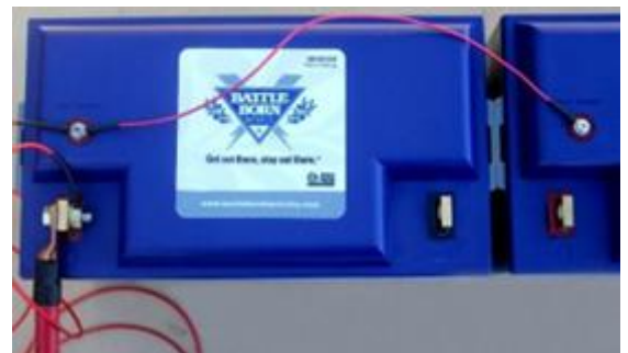
Figure 7: Top view of daisy chained heat-enable post
