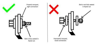
Figure 2: Proper and Improper Terminal Connections
