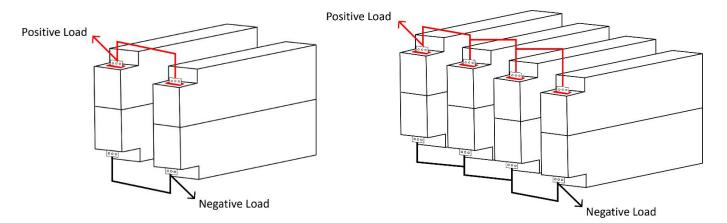
**Figure 3.1:** Two GC3 Batteries connected in Parallel to create a 12V 540Ah Battery Bank
