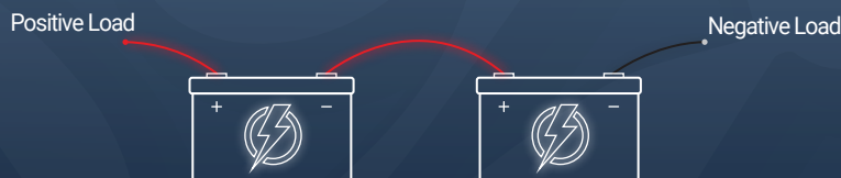
Series Connection 24V 50Ah Bank Increases Voltage, Ah stays the same.
