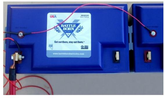
Figure 7: Top view of daisy chained heat enable post
