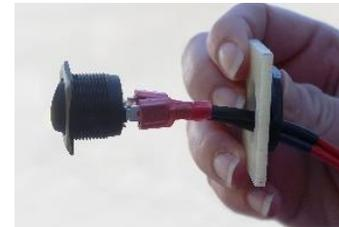
Figure 10: Heat Battery Kit harness connected to rocker plastic nut from rocker switch
