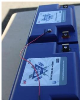
Figure 6: Side view of daisy chained heat enable post
