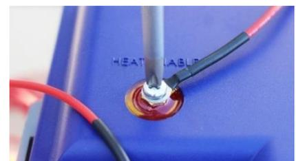
Figure 13: #8 ring terminal onto the heater enable post
