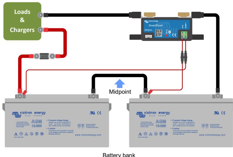
For more information on midpoint monitoring see chapter 9. This chapter also provides information and wiring diagrams on how to monitor the midpoint of battery banks that have been wired in series/parallel.
