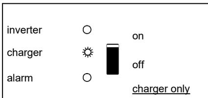
The AC input voltage is switched through and the charger operates in float mode.
