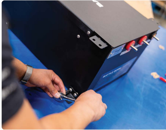
Images 4 & 5 Installing Mounting Brackets
